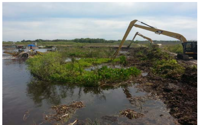
FWC staff utilize a harvester to mechanically remove floating tussocks in Emeralda Marsh.
