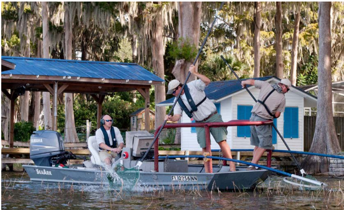
Electrofishing boats use a generator and sophisticated electronics to create a current that stuns fish, allowing biologists to net them.
